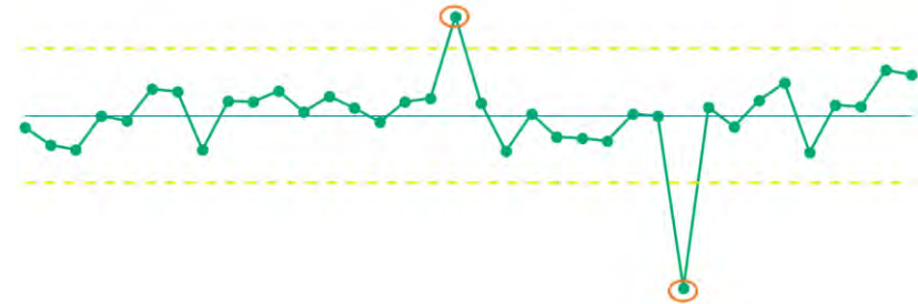
Rule 1: Single data point outside the control limits
